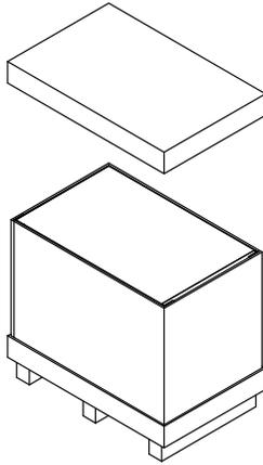
Remove the top of the shipping container to expose the rack unit.
