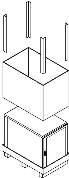
Remove the shipping container from around the rack unit by removing the corner supports and lifting the shipping container sides from around the rack unit.
