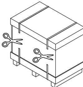
Cut away and remove the securing straps on the outside of the shipping container.
