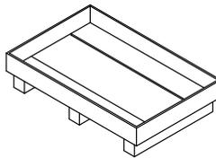
Lift out the rack unit from the shipping container base. Take care not to damage the rack unit when removing it from the base.
